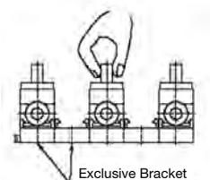
Figure2 Manifold piping with the lever turned around by hand
